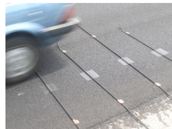
Figure 6. Pneumatic road tubes. TSC for surveys.
