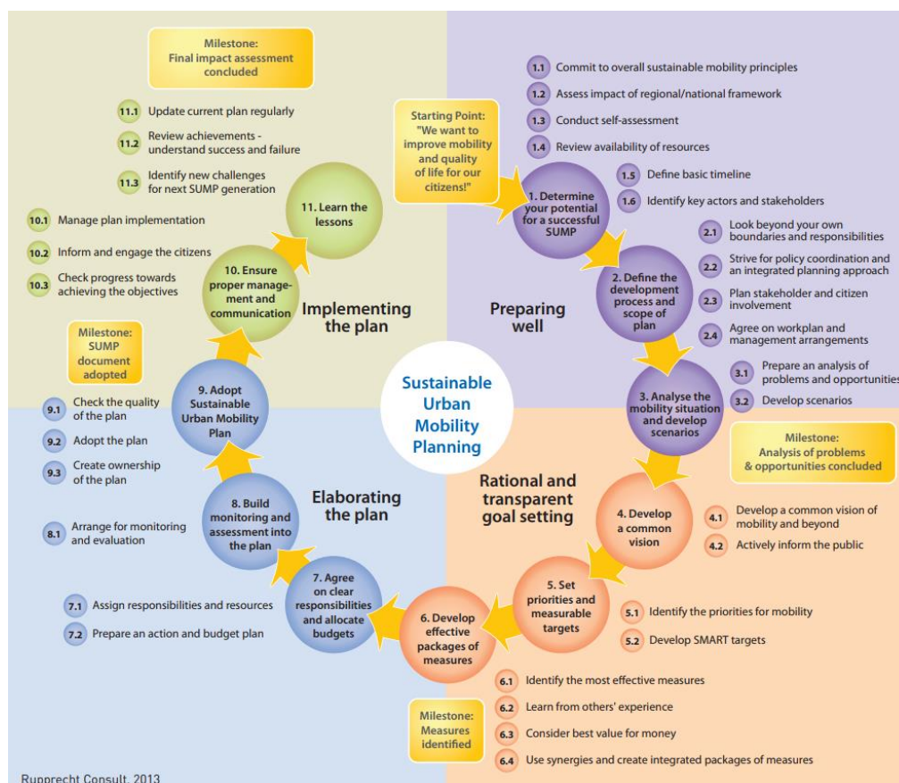
Figure 3. Planning cycle for a sustainable urban mobility plan. Guidelines: Developing and implementing a Sustainable Urban Mobility Plan
